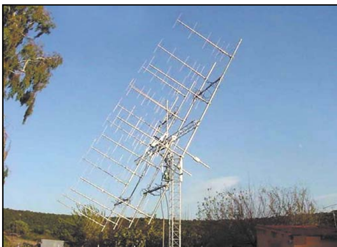
The 2-meter array (16x6 cross-polarized, 1.1 wavelength, 22 dBd) of Jimmie, SV1BTR.
